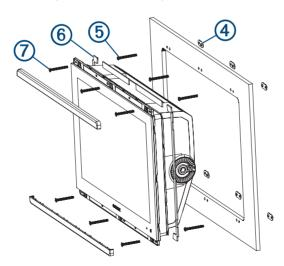
8 Secure the nut plates to the mounting surface by fastening the pan head machine screws 5 through the holes with the raised portion of the nut plate.
